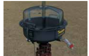
The Trapper Topper installed with a float switch and drain valve
